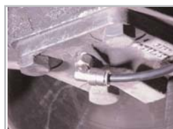
Practical example, king pin: usually 4 lube points
