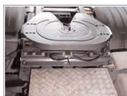
Practical example, fifth-wheel support plate: usually 6 lube points
