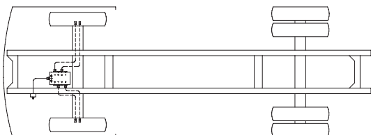
Practical example, king pin: usually 4 lube points
