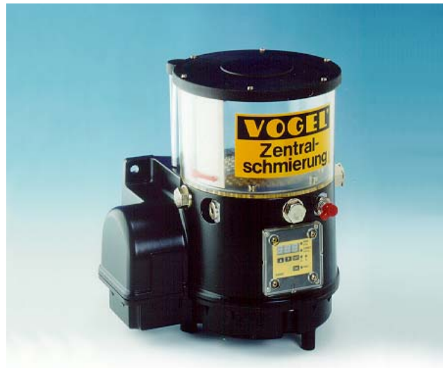
KFGS1-5 2-liter reservoir capacity
