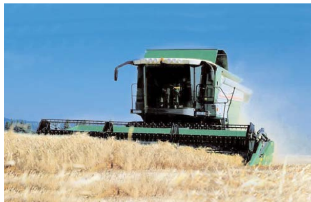
Combine harvester with progressive central lubrication.
