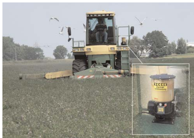
KFGS3-5 installed on a self-propelled mowing machine.
